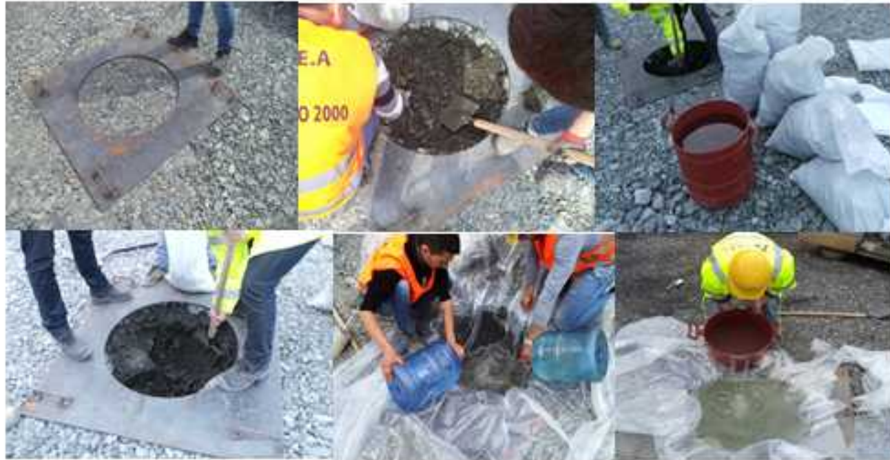
Procedure of determining field density measured by water replacement method
