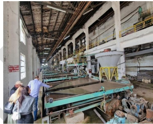
Figure 11 - Gravity separation is often applied, as chromite has a higher specific gravity than surrounding waste material.
